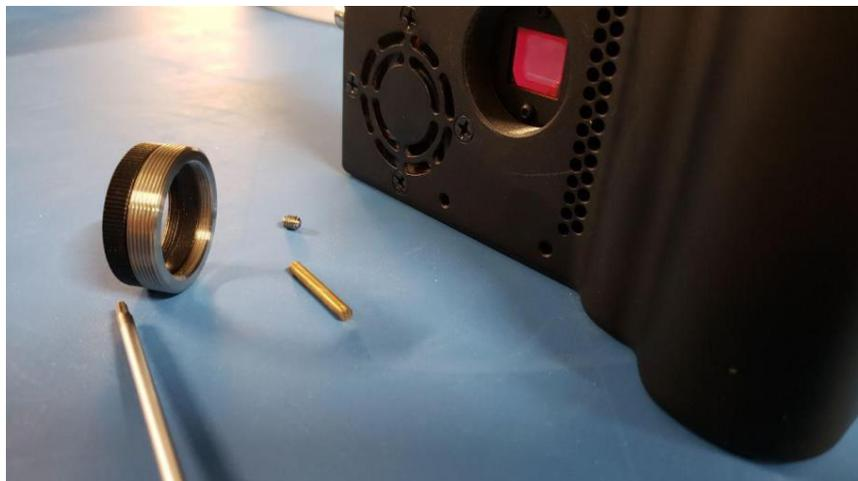
2. Loosen the two IR frame screws and carefully remove the frame without scratching the filter. Note that the filter is extremely sensitive and even the lightest touch can scratch it.
